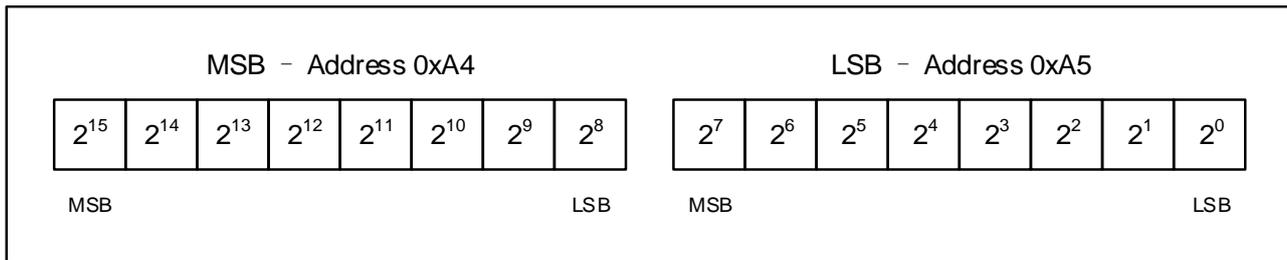
Figure 16. CYCLECNT Register Format
