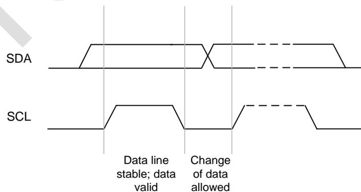
Figure 20. Bit Transfer on the I2C Bus
