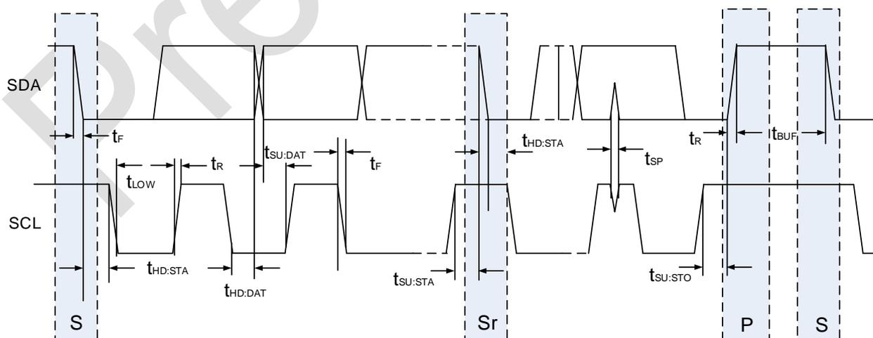
Figure 2. I<sup>2</sup>C Timing Diagram
