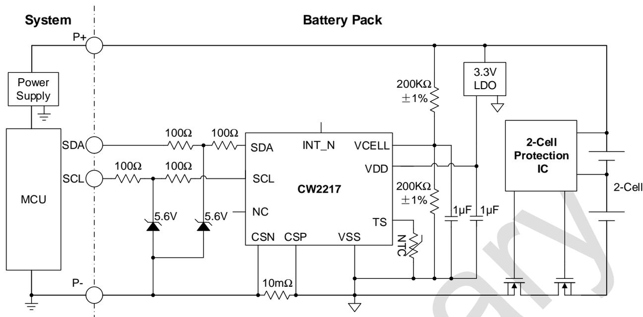
Figure 28. Typical Application for 2-Cell Pack Side
