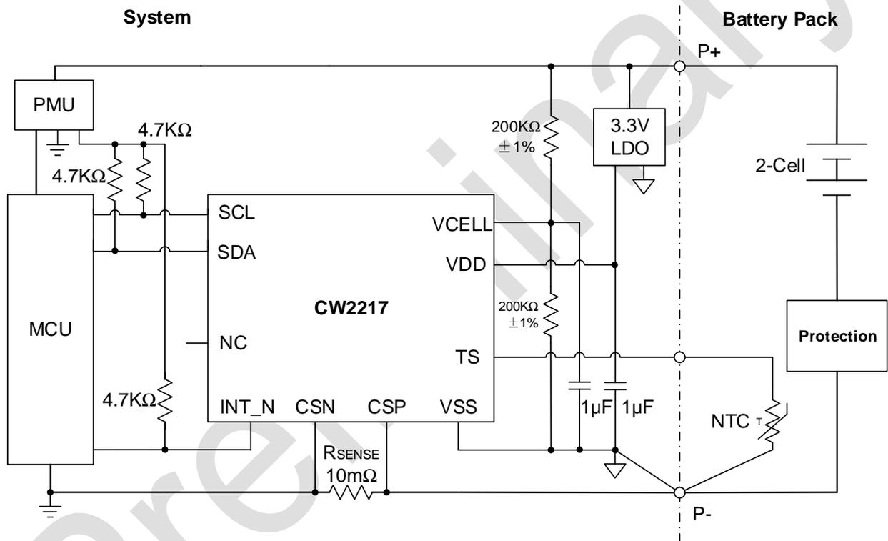
Figure 27. Typical Application for 2-Cell System Side
