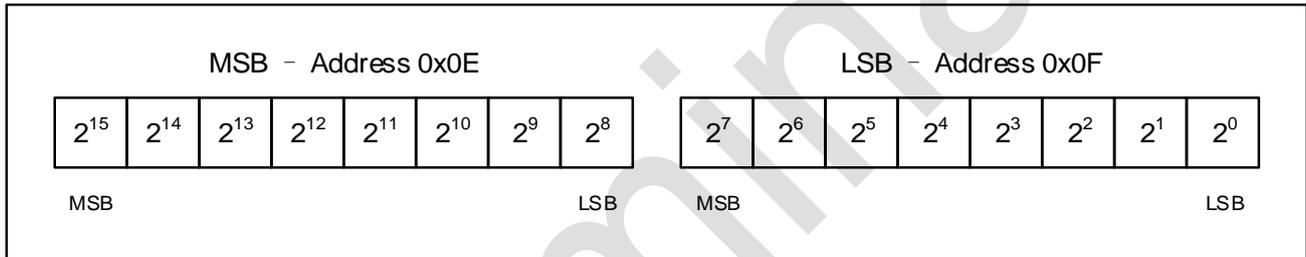
Figure 13. CURRENT Register Format
