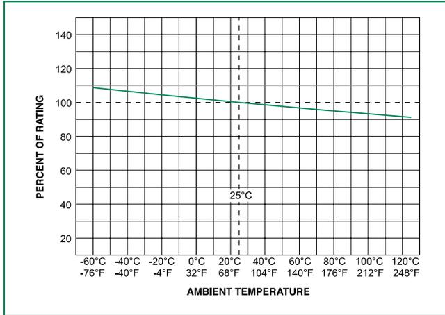
Notes: Derating depicted in this curve is in addition to the standard derating of 25% for continuous operation
